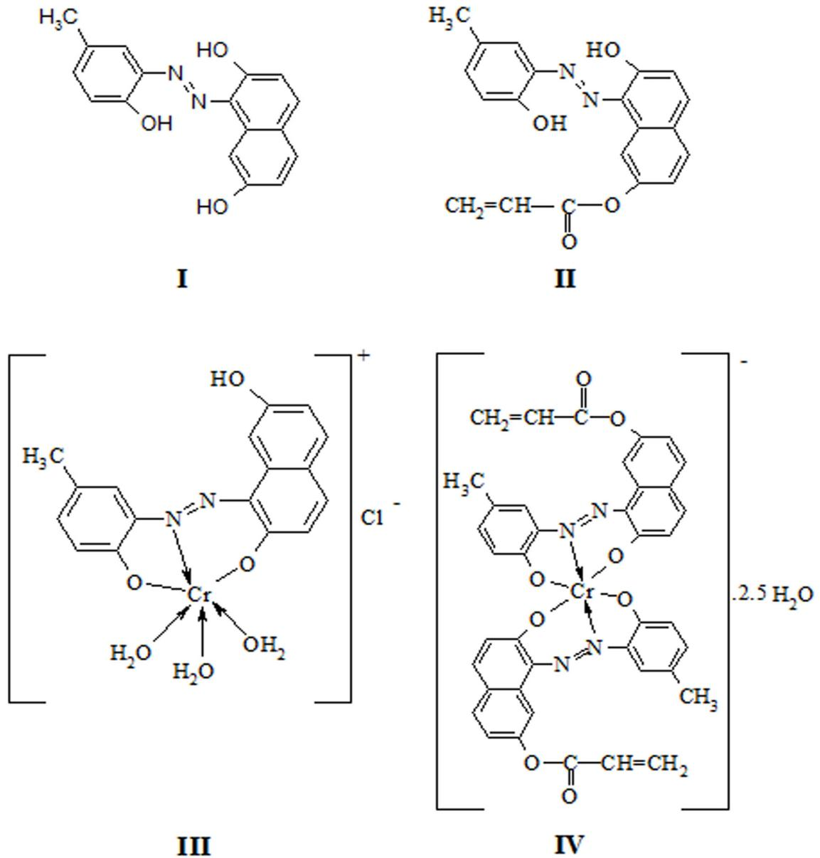
**Figure 1.** The structure of the 7-hydroxy-o,o'-dihydroxyazo dyes and their chromium complexes.
