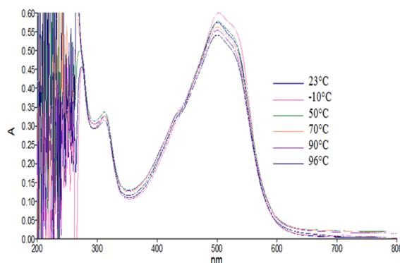
**Figure 6.** Absorption spectra of dye II ( $5 \times 10^{-4}$  M) at different temperatures DMF.
