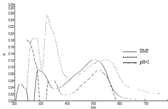
**Figure 3.** Absorption spectra of dye I ( $1 \times 10^{-5}$  M), pH 2 and pH 12 in DMF
