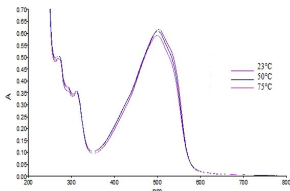
**Figure 5.** Absorption spectra of dye I ( $5 \times 10^{-5}$  M) at different temperatures in ethyl alcohol.
