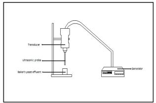
Fig.1. Schematic diagram of the ultrasonic reaction system
