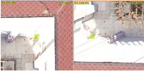
Figure 11. Challenges acquiring data from photogrammetric model. Shadow of the manmade structures and/or vegetation may prevent a proper positioning. At DC5, shadow of vegetation around the corner partially block the view and makes it harder to assess the actual location. Green cross represents the estimated location and yellow circle is the error estimation for the point.
