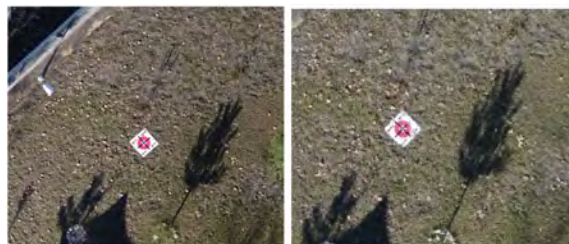
Figure 9. One of the temporary GCPs established on the ground for each flight. Image on the left is from actual photo of the feature and the right one is obtained from densified point cloud.
