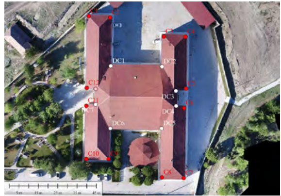
Figure 7. Main structure at the center of the campus from above. 12 red dots are regular corners (C), and 8 white dots are deep corners (DC).
