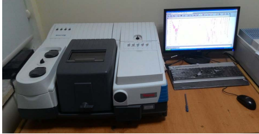
Resim 3.5. FT-IR (Fourier Transform Infrared) spektrometresi
