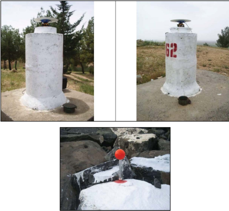
Figure.3. Pictured at the top are the reference stations with GNSS equipment. Below them is the object point with a target for angle measurement.
