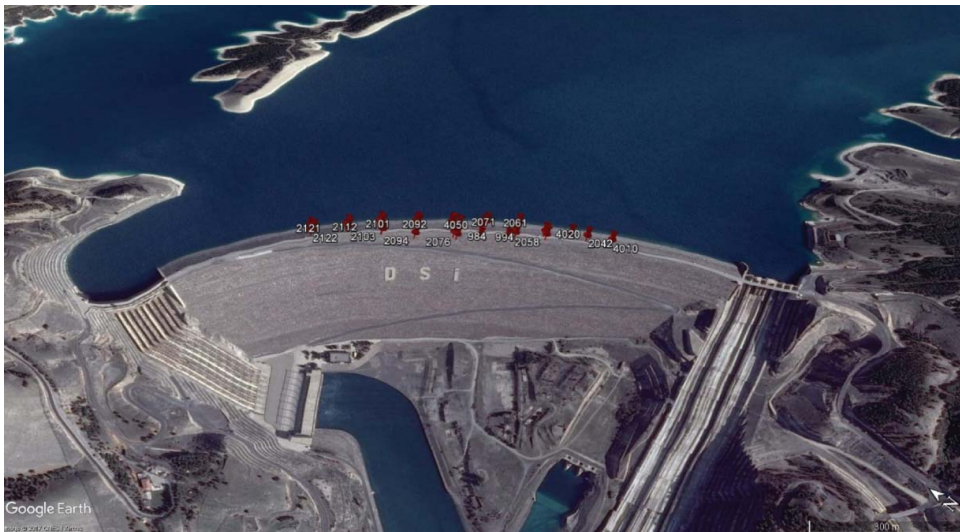
Figure 4. Location of the 30 object points having maximum displacement vectors.
